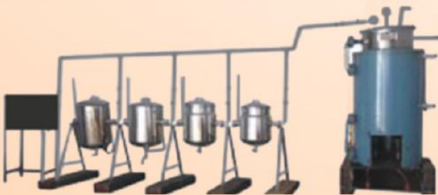
Steam Boiler Setup
