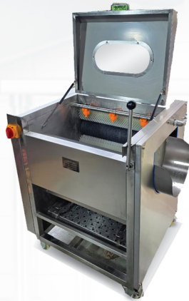
Automatic Root Vegetable Peeling Machine (Brush stone Hybrid Model)
